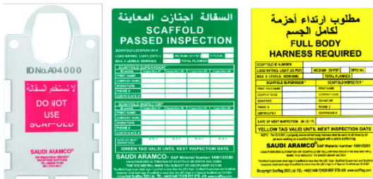
Figure G. Scaffold Inspection Tags (Red, Green, and Yellow)
